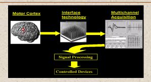
Fig.4 Brain-to- Machine Mechanism
